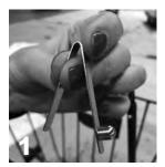
Squeeze both open ends of the pin while you place it in the arm of the basket until the little knob pokes through the hole.
